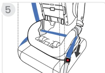
6. **Remove** slack from the lap part (a), then the shoulder part (b) of the vehicle belt.
