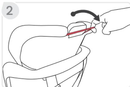
3. **Route** the harness through the head restraint cover slots.
