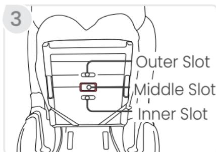
4. **Turn** the buckle strap retainer sideways and **push** it through the seat pan slot, the seat pan cover, and the positioning layer, if necessary.
