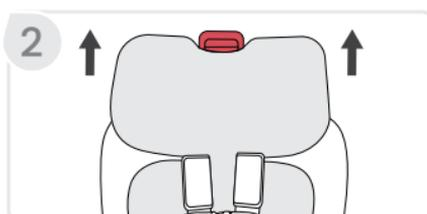
3. Gently **pull** head restraint on each side to ensure it has locked into position.
