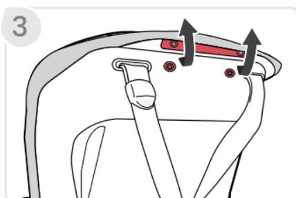
4. **Untuck** the plastic tabs under the forward-facing belt path on each side.
