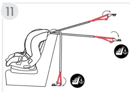
12. **Pull** the loose tether strap end to remove slack and **secure** excess webbing with the tether storage strap attached.
