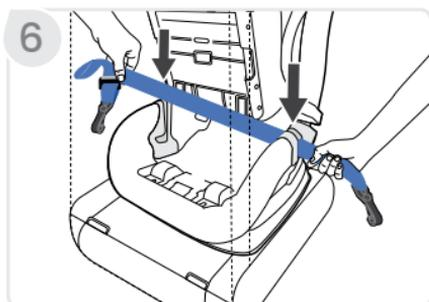
7. **Firmly** press the lower anchor attachment **over** their adjacent lower anchors.
