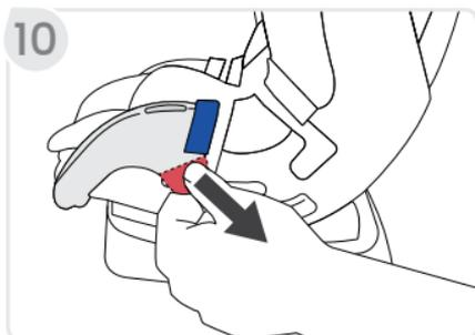
11. **Detach** the two (2) elastic straps at the bottom of the child restraint.
