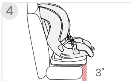
**NOTE:** Ensure that no more than 3" (7.6 cm) of the base hangs over the edge of the vehicle seat (see page 12).
