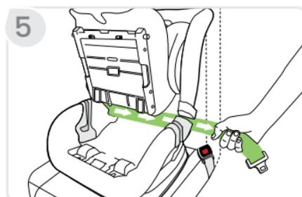
6. **Buckle** the vehicle belt. **NOTE:** Ensure the vehicle belt is not twisted.
