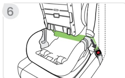
7. **Push** down into the vehicle seat bight with moderate force (approx. 45 lbs/20.4 kg), compressing the vehicle seat while tightening the vehicle belt.
