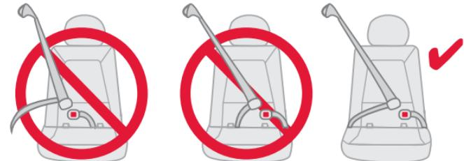
Lower anchors can be used to secure the child seat to the vehicle seat even when unoccupied, since in a crash an unsecured child restraint system may injure occupants. Secure your child using the vehicle's lap-shoulder belt system.
