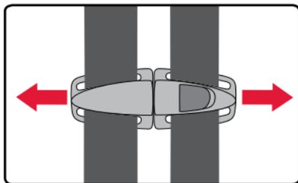
4. Release the buckle and attach the harness straps to the harness holders.
