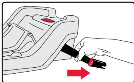
3. Place the base on the vehicle seat and press the lower connectors onto the adjacent vehicle lower anchors until a click is heard.
