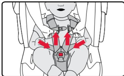
9. Slowly pull the adjuster strap to tighten the harness around the child.
