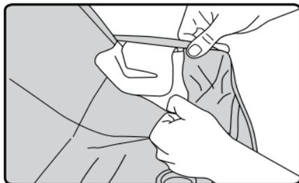
6. Pull cover from around harness adjust button and lift the seat cover away from the seat shell.
