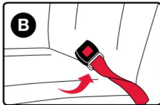
**Possible solution:** Adjust the infant car seat base to a higher position to avoid any potential interference with the vehicle belt buckle. Ensure that the infant car seat recline indicator is in an allowable position once installed.
