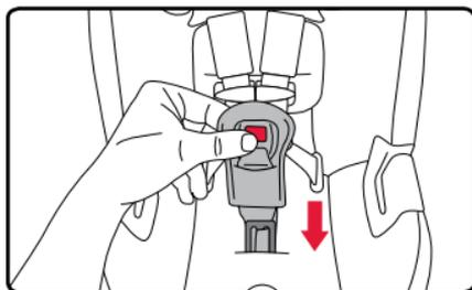
6. Pull up on the buckle to ensure that the buckle strap retainer is properly seated.
