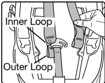
1. Loosen the infant car seat harness by pressing the harness adjuster release button and pulling both harness straps forward.
