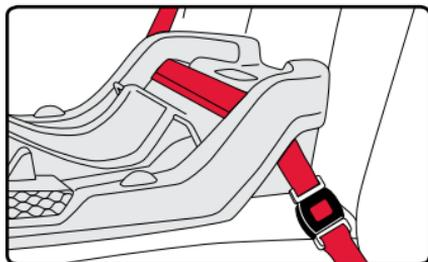
3. Press the base firmly into the vehicle seat while removing all slack from first the lap portion and then the shoulder portion of the vehicle seat belt.
