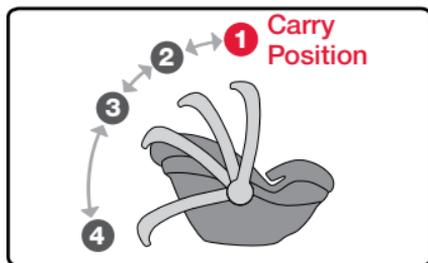
To adjust, press and hold both handle adjuster levers and rotate the handle to the chosen position.
