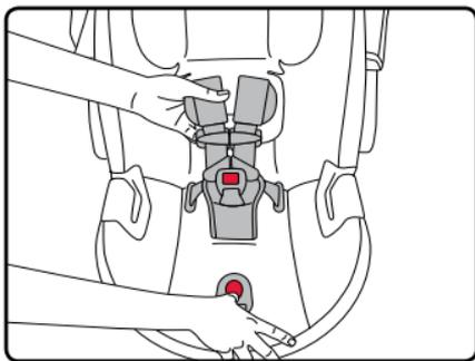
2. On the back of the seat, squeeze the harness height adjuster and slide the harness to the appropriate height.
