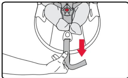
**NOTE:** *Snugly adjust the belts provided with this child restraint around your child. A snug strap should not allow any slack. It lies in a relatively straight line without sagging. It does not press on the child's flesh or push the child's body into an unnatural position. You should not be able to pinch excess.*
