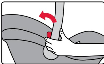
**IMPORTANT:** Do not force the carry handle past the upright carry position toward the child's feet. Doing so may cause damage to the carry handle.
