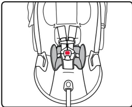
Option 2: Provides additional support behind your child to achieve head and neck alignment. To use, rotate the comfort pillow 180 degrees from the shipped position and tuck behind the bib of the head restraint cover.
