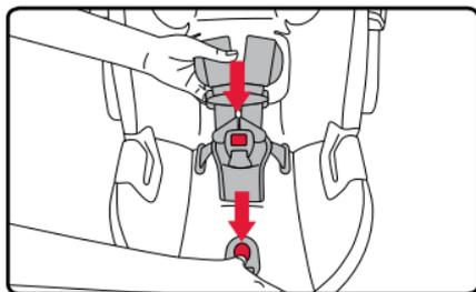
3. Press the tab and pull apart the two halves to release the chest clip.
