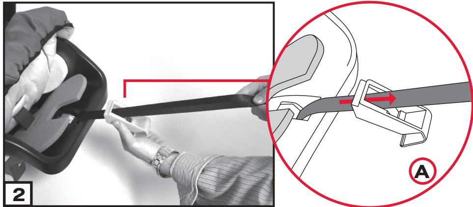
3. Angle the harness adjuster retention clip down over the release button assembly until the top of the clip is seated under the edge of the shell.
