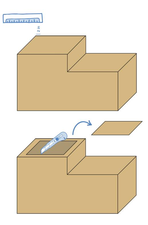
Divide the rectangle you took out into 3 parts (making half cuts), fold it into 3, forming a "tube" and set it aside.
