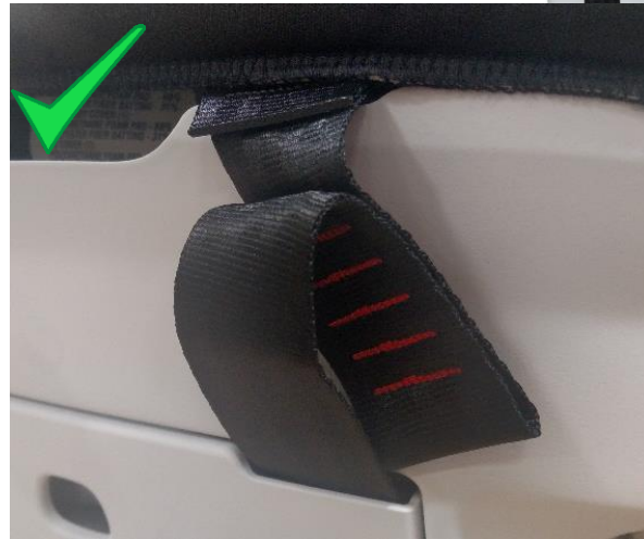
Change in manufacturing: Sewn loop with red lines visible
